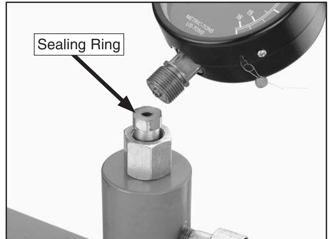
Figure 16. Hydraulic line installation.
